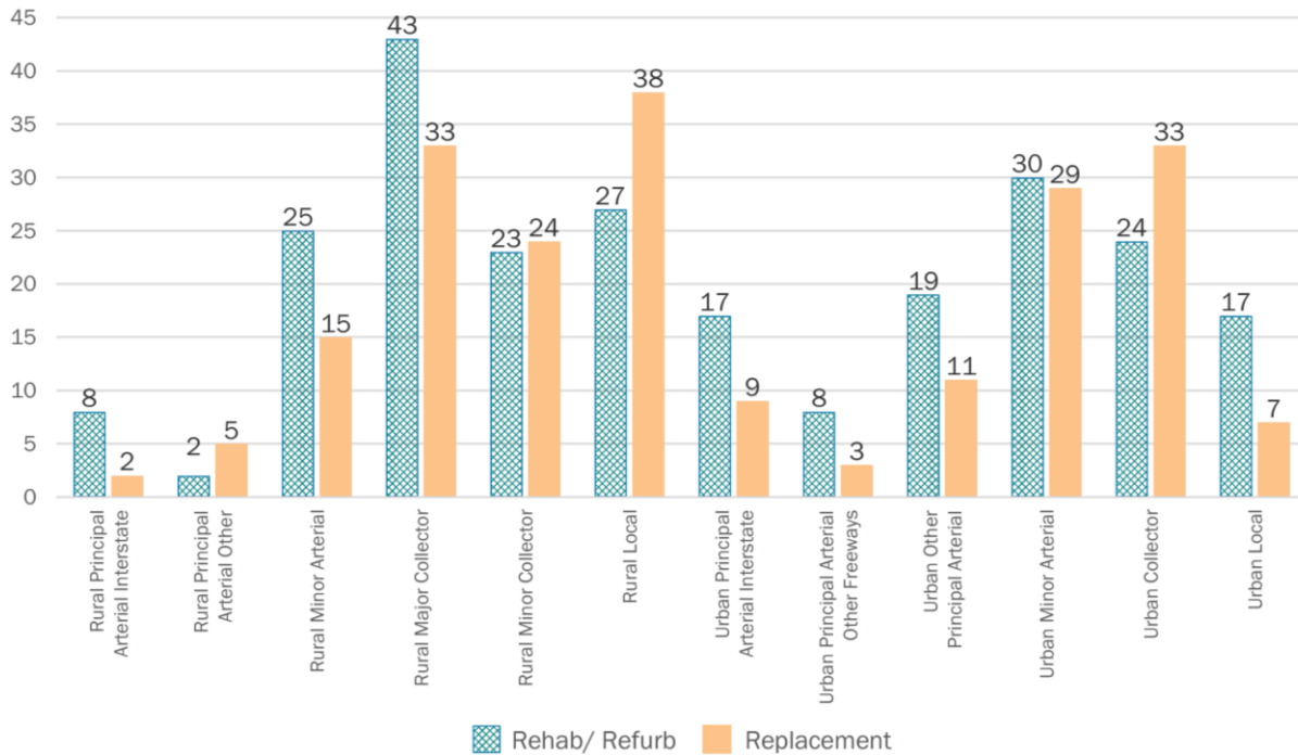
Figure 25: Distribution of Bridges in Need of Rehabilitation/Refurbishment or Replacement, by Functional Class
